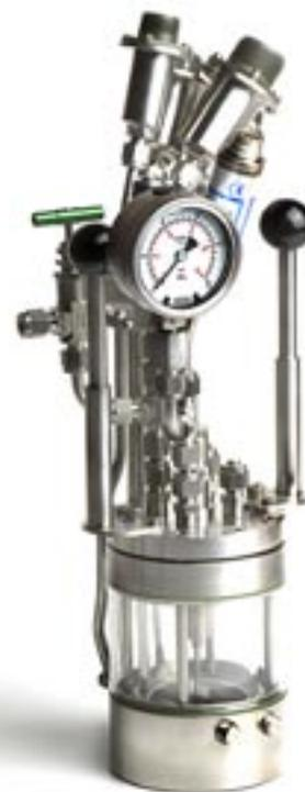
The standard reactor is a cylindrical, double walled glass vessel. It is capped, top and bottom, with stainless steel. Its special design makes it very handy for the operator. The open vessel can be placed on a balance during the charge of solvents, chemicals etc. The reactor lid holds the shaft seal and the necessary armature for safety and for charging, evacuation, sampling etc.
