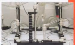
New volume change adjustments provide quick and easy volume settings from 250ml to 1000ml in 50ml increments. Fill 6 or 7 flasks in Hanson, VanKel, Distek, Erweka or other baths.
