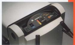
New operational panel provides easy-to-use controls. One simple button initiates complete media measurement/deaeration/dispense cycle. Fills the dissolution bath in 3 minutes.
